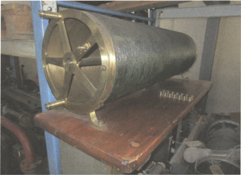
Figure 3.9: The original Lorenz machine in its improved form kept at the Danish Museum of Science and Technology in Elsinore. The brass cylinder of length 1 m and diameter 0.3 m is wound with a single layer of thin copper wire. The cylinder was rotated by an electric motor with a frequency of 250 per minute and connected directly to the shaft of the cylinder. Published with permission of the Danish Museum of Science and Technology.
